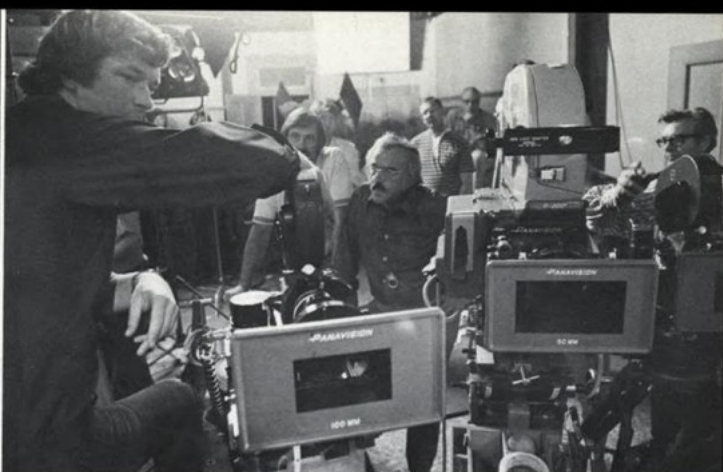
(LEFT) For a follow shot of Brynner walking down a corridor, fill illumination was provided by bounce light from a one-inch-thick sheet of styrofoam measuring 48 x 48 inches. A PAR-64 "six-lite" lamp was used as the light source. (RIGHT) Three cameras are set up for a multiple-camera shot. Despite increased expense of additional cameras and operators, considerable money was saved by this method, because costly and time-consuming stunts did not have to be repeated to achieve a variety of angles.
